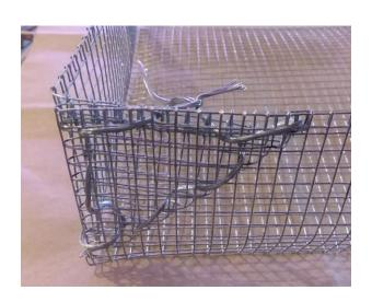
8a. Weave the wire through the tab and the basket around the perimeter so the two ends meet at the top.
