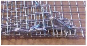
9a. Twist the two ends together, cut off the excess and push the tab flat against the side of the basket. All of this will get covered in tape and won't stab the user.
