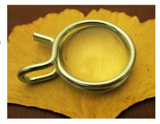
The lens is borosilicate glass used for low-watt LEDs, like flashlights. They are available for about a dollar each on eBay.com. I've carried one in my pocket for about a month now, along with change, keys, metal stuff I pick up off the ground, etc. and it hasn't scratched or scuffed.
